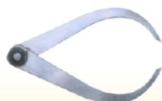
Firm Joint Out Side
